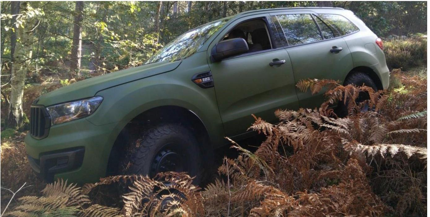
***The VLTP-NP, 3.5 tonnes, 150 CV, a carrying capacity of 900 kg***
