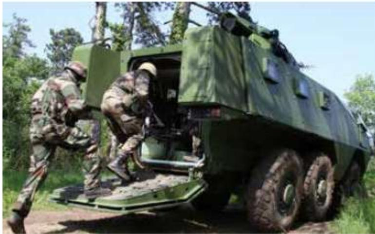
Mack Defense provides the **LAKOTA**, an armored medium vehicle 6x6 offering high level performance in terms of mobility, protection and payload. Equipped with a 370 hp engine coupled with an automatic transmission, the LAKOTA is a multirole vehicle and can receive a large equipment range,
