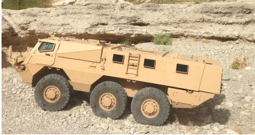
The VAB Mk. III is an infantry armoured vehicle available in several versions.
