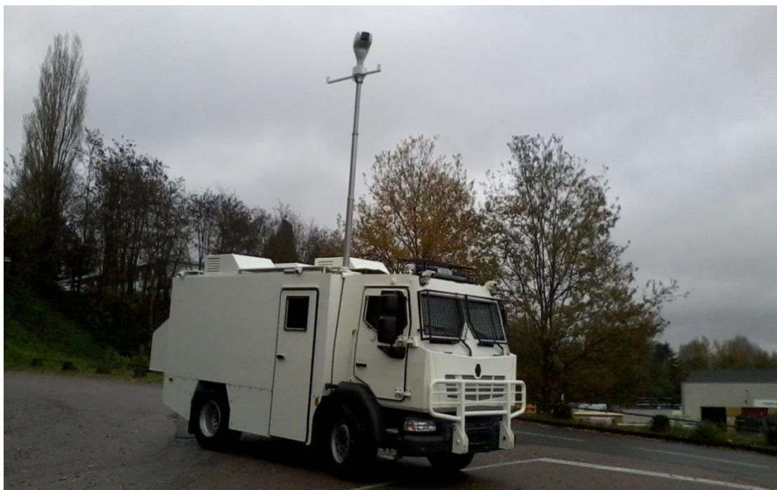
*A 360° swivelling camera fitted onto a deployable mast ensures long-range observation*
